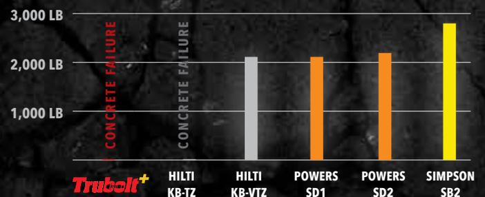
\*Performance comparison of 3/8" wedge anchors on 2,500 concrete PSI: ICC-ESR 3772, 1917, 3904,3037,2818,2502.
